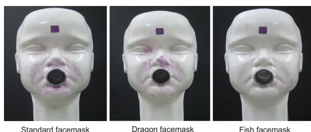
Figure 8. Face model after droplet deposition at moderate inhalation.
