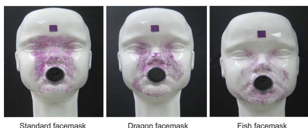
Figure 7. Face model after droplet deposition at shallow inhalation.
