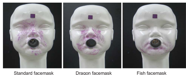
Figure 5. Face model after droplet deposition at 10 L/min.
