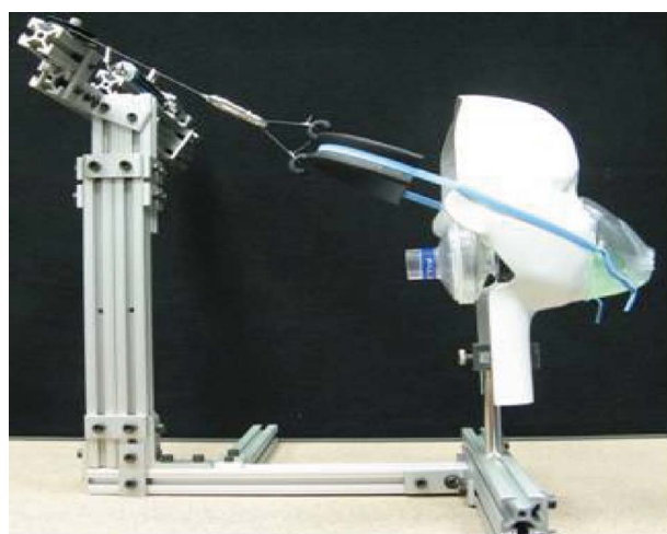
Figure 1. Experimental apparatus for standardized assessment of facial and ocular deposition.
